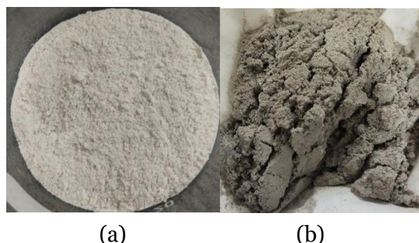
Figure 3. Isolation results of silica ( \text{SiO}_2 ) with HCl (a) with aquades washing; (b) without aquades washing
