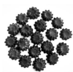
Gambar 13. Pellet Besi Hasil Proses Microwave
