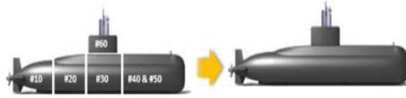
Figure 2. The Third Submarine (KRI Alugoro-405) Joint Section from the First Batch
